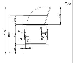
Electric Supply voltage: 220-240 V/1N ph/50/60 Hz Electrical power, max: 2.04 kW Water: Water drain outlet size: 3/4" **Key Information:** N° of doors: External dimensions, Width: 770 mm 1180 mm External dimensions, Depth: External dimensions, Height: 1304 mm Net weight: 94.5 kg Shipping height: 1420 mm Shipping width: 910 mm Shipping depth: 830 mm Shipping volume: 1.07 m<sup>3</sup> +85 / +9<u>5</u> °C Set temperature:
